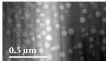
Figure: Nanocomposite morphology (A2 nanoparticles in a B2 matrix) of  $\text{Al}_{28}\text{Co}_{20}\text{Cr}_{11}\text{Fe}_{15}\text{Ni}_{26}$  as visible in HAADF-STEM.
