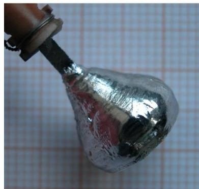
Fig. 2:  $\text{In}_7\text{Pd}_3$  single crystal grown from an In-rich solution of  $\text{In}_{86}\text{Pd}_{14}$  composition. (mm grid)
